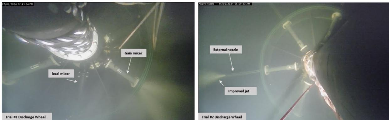
Figure 11: Discharge wheel in the first (left) and second trial (right) following modifications to increase the velocity and spread of the discharge jets.
